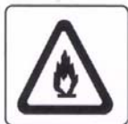
WARNING - Flammable liquid.
