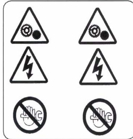
WARNING - Do not undertake any maintenance on this machine until the electrical supply is disconnected and the air pressure is totally relieved.
