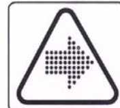
Air/gas flow or Air discharge.
